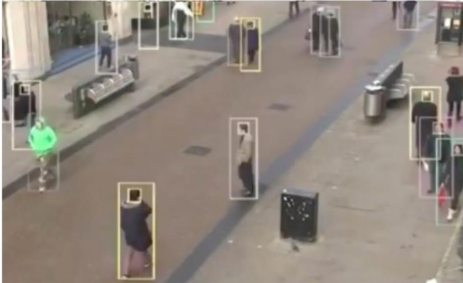
Finally, this is a sequence of frames in a video where the green person is successfully tracked from frame to frame. Further, the other individuals are all tracked showing that the SIFT algorithm is useful in tracking multiple features (blobs) in images simultaneously.
